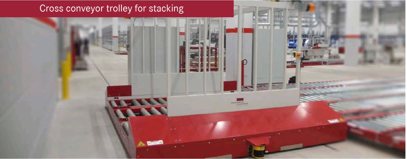
Cross conveyor trolley with lifting mechanism for stacking
