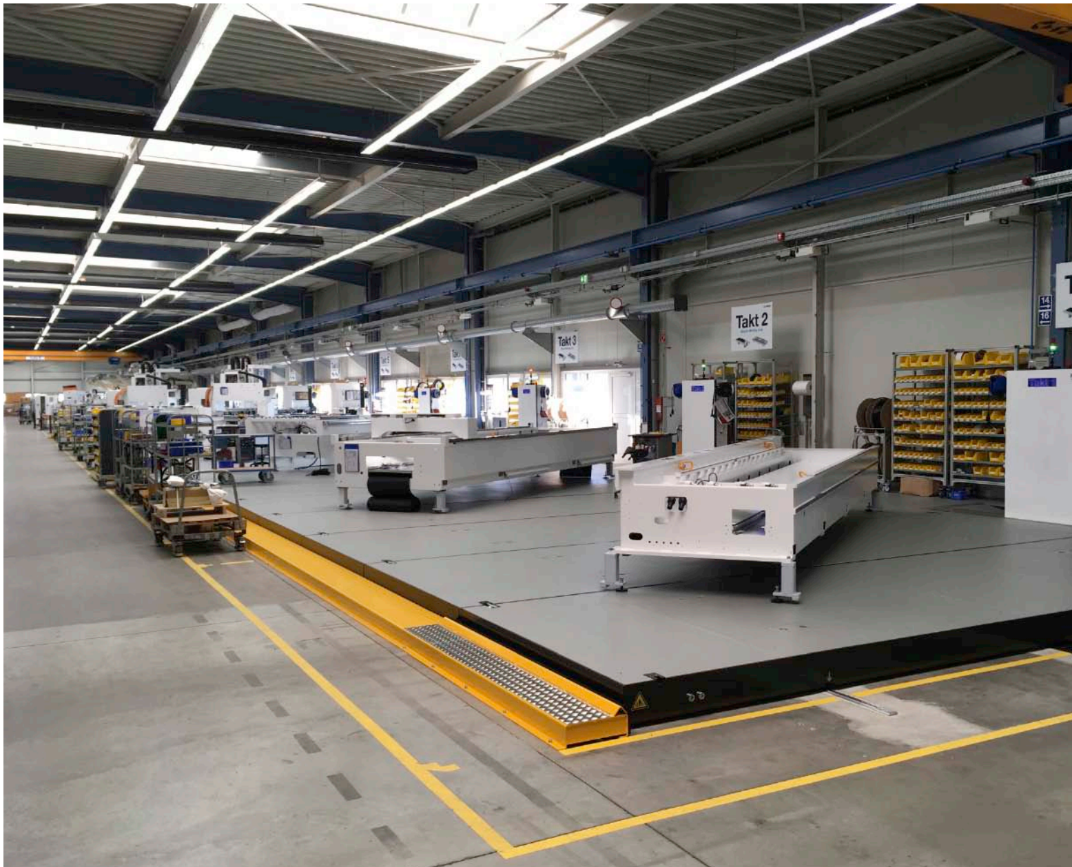
Assembly line with central cycle drive for the synchronous feed of all assembly stations
