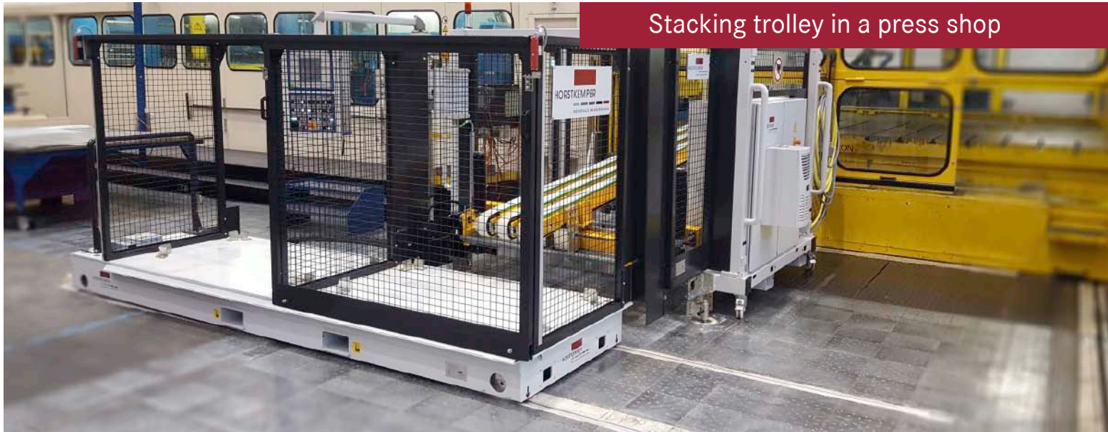
55 tons - die transport trolley
